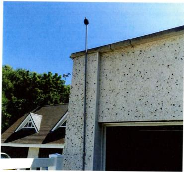
Figure 3: Noise Logger Setup
