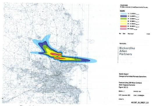
Figure 6: DAA predicted LAeq,16hour (07:00 - 23:00) airport noise contours for 2025.
