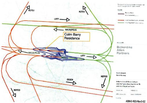
Figure 8: Predicted LAGG. 15hour airport noise contours with North Runway in operation.
