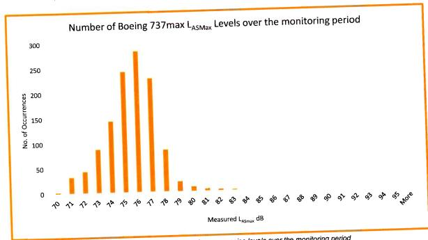
Figure 15: Number of Boeing 737-max LASmax, 1mm noise levels over the monitoring period
