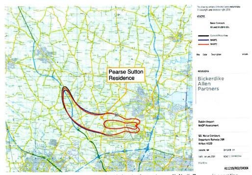
Figure 11: Predicted Sound Exposure Level airport noise contours with North Runway in operation.
