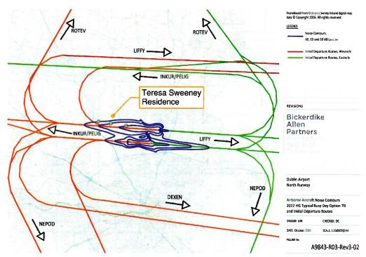
Figure 5: Predicted L<sub>Aeq,16hour</sub> (07:00 – 23:00) airport noise contours with North Runway in operation.
