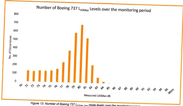
Figure 13: Number of Boeing 737 LASmax 1min noise levels over the monitoring period
