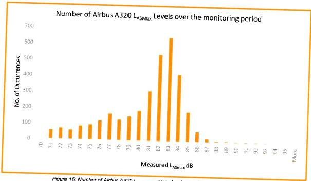
Figure 16: Number of Airbus A320 Lasmax, Imm noise levels over the monitoring period
