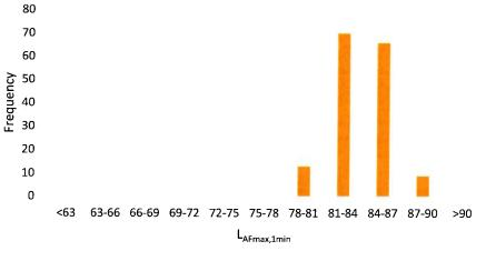
Figure 6: L<sub>AFmax</sub> noise events for Boeing 737
