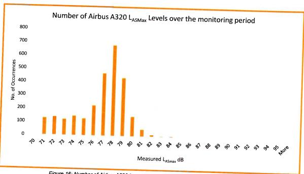
Figure 16: Number of Airbus A320  $L_{ASmax\ 1min}$  noise levels over the monitoring period
