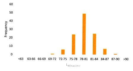
Figure 5: L<sub>AFmax</sub> noise events for Airbus A320
