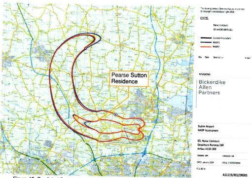
Figure 12: Predicted Sound Exposure Level airport noise contours with North Runway in operation.
